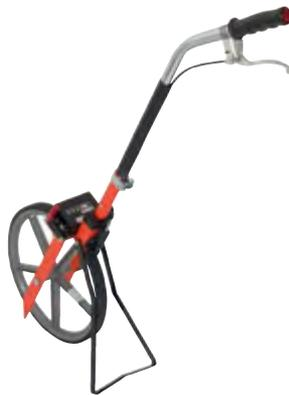
Measuring wheel with hand brake
