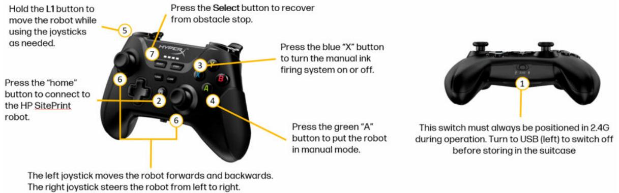
The controller is used to manually control the robot to ease the movement between areas, to position it to start a job or to help the robot to overcome a certain obstacle.
