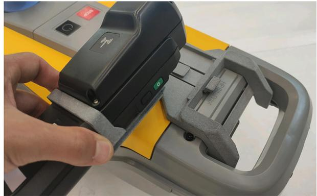
5. Press the button to allow it to slide fully in.
