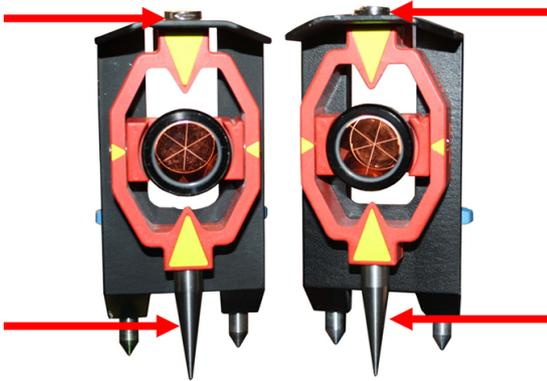
2. Rotate the leveling screws left or right to level the bipods.
